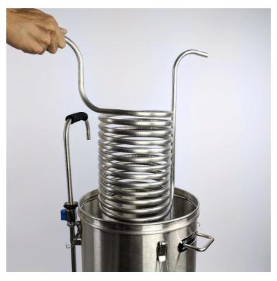
Although the immersion cooling coil was intended to be used with cold water running through it there is also another method that is worth mentioning. That is to run the hot wort through the coil then to immerse the coil into an ice bath.
