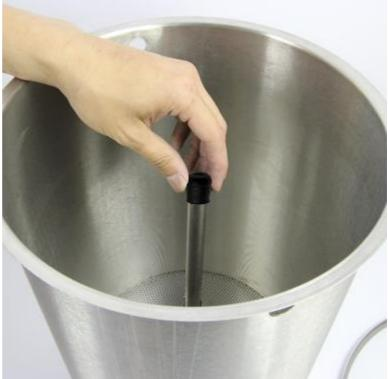
We recommend installing the malt pipe handle before you add your grain and malt pipe
