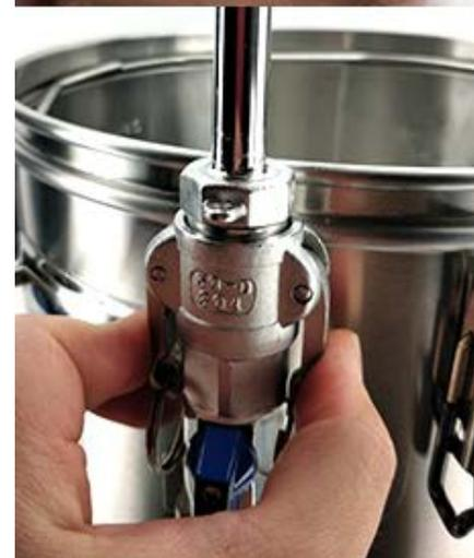
switch off the pump and readjust the camlock to the position you need then re-engage the camlock.
