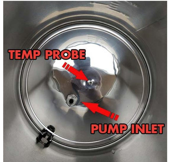
The photo to the right shows the placement of the probe. The probe placement has been designed like this as it prevents the element from overheating and scorching wort by taking the temperature of the wort closest to the element. This is why your strike temperature needs to be accurate!
