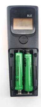
Once the batteries have been installed the device should beep and the screen should automatically power on.
